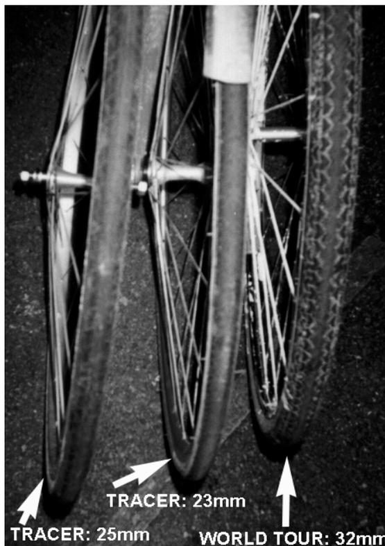
The three pneumatic tyres used in this experiment were all made by Michelin. The World Tour has a chunky tread whereas the Tracers have a thinner smooth rubber wall with a tread of thin cuts which are not visible in this slightly defocused photo.
